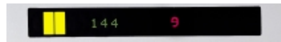
On the left, the green figure indicates the number of passengers. On the right, the red figure shows the number of alarms.
